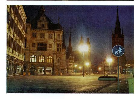
Moreover, the county town Halle has an imposing traffic-free zone ending in the historical market-place. This borough is illuminated by means of post-top fixtures with the NA 175-01 lamp type. The fixtures are arranged in groups of 18 units mounted on the top of steel posts of 8 m in height (Fig. 18).
