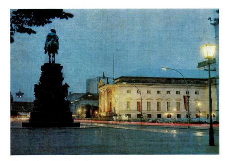
Fig. 9 demonstrates the pedestrian area illuminated by polemounted post-top fixtures equipped with high pressure sodium lamps NA 70-01. The fixtures are mounted on steel poles of a height of 3.5 m staggered on both sides.
